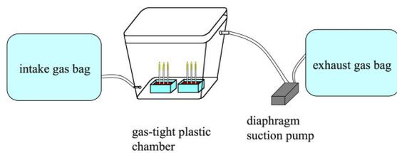
**Fig. 1.** A schematic illustration of the experimental system for the supply and replacement of ethylene-containing air.
